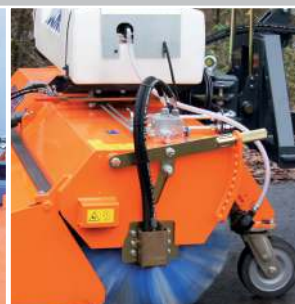
Adjusting-lever system with optimized sweeping-angle
