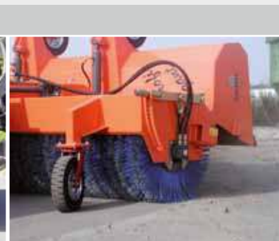
easy brush adjustment by adjusting-lever system
