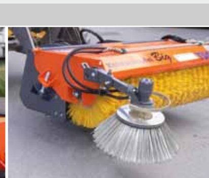
fully adjustable hydraulic side brush (50% PP / 50% wire)
