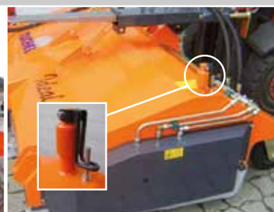
Brush adjusting lever facilitates brush adjustment
