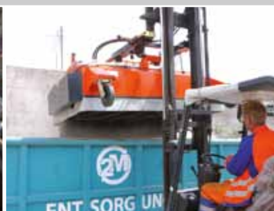
Hopper incl. hydraulic tip (standard)
