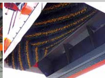
Special V-brush for sticky and fine dirt
